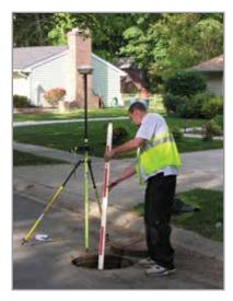
equipment to collect data to survey grade or centimeter level accuracy. Following the completion of the verification effort, SSA trained Department staff to use the handheld GPS equipment, specifically the Trimble ProXH GeoExplorer with GPS Analyst post processing.
